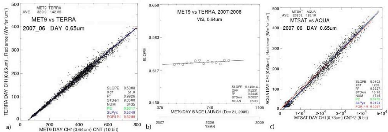
Fig. 1. Correlations and regression fits between (a) *Meteosat-9* and *Terra* MODIS VIS channels and (c) MTSAT-1R and *Aqua* MODIS VIS channels, June 2007. Standard linear fit in black, principal component fit in green, reversed axis linear fit in blue, and force fit to zero or known space count in red. (b) slopes of linear regression fits between *Meteosat-9* and *Terra* MODIS VIS channels.
